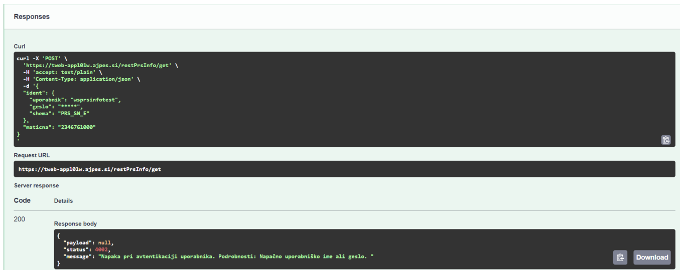
Picture 1: An example of a restPrsInfo REST API response (GET method) – User authentication error. The input message contained an incorrect password '*****'. Since there is no business data, the payload field is NULL.
